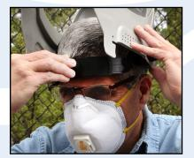
4) Press adjusting knob inward to engage mechanism, and rotate knob clockwise to tighten head strap to desired fit and comfort level.
