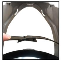
**6)** The strap on the crown of the head is also adjustable, and for most users adjusting this strap is not necessary. To adjust the crown strap, remove the helmet and rotate internal head strap to allow access to crown strap. Disengage the two parts, adjust as desired and reengage the two parts.
