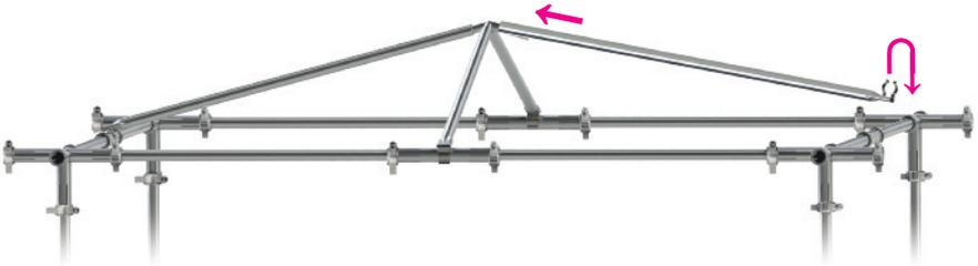
**TIP:** It is recommended to first slide the Ceiling Poles over the Four-Way Hub with the clips facing up. Once the Ceiling Pole is attached to the Four-Way Hub, rotate the pole so that the clip faces down. Snap the clip over the Straight Union.
