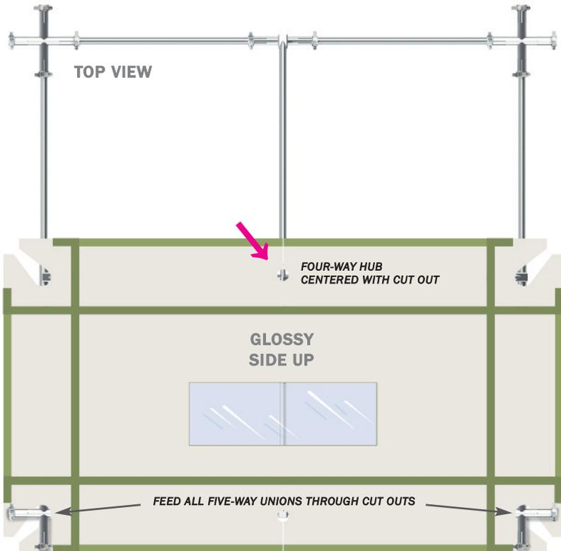
**NOTE:** The wall and ceiling framing can be assembled prior to hanging the Wall Panels, or the ceiling framing can be added after the Wall Panels are hung. It is recommended to have the Wall Panels hung prior to adding the Ceiling Panels. The wall's hook and loop fasteners secure the first Ceiling Panel's position, then making it easier to correctly position the second Ceiling Panel.
