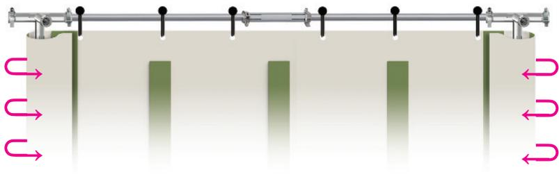
**NOTE:** There should be no gaps between joining wall panels. If the edges of two walls don't hook and loop together, un-wrap one of the poles, and hook and loop the pole in the opposite direction.
